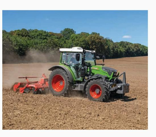
The heart and soul of every Fendt tractor is its Vario® CVT transmission. The stepless Vario CVT, with no clutch packs, optimizes engine power and fuel economy, with seamless travel from 65 ft/h to 25 mph. Operate in either joystick or pedal mode for the ultimate driving experience.
