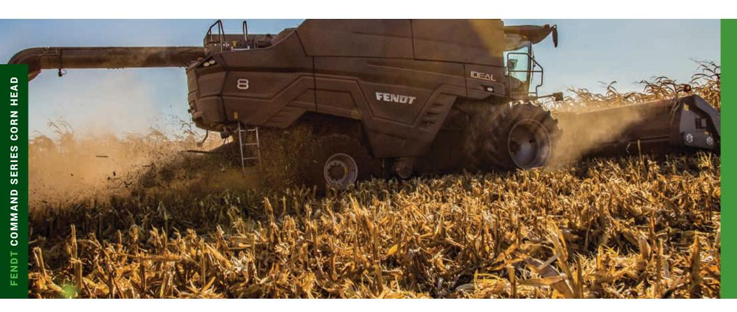
Residue Management—Available in chopping or nonchopping models, the 3300 Command Series headers promote exceptional residue management for your farm. The stalk rolls designed with point-to-point knife contact increase aggression, which increases overall effectiveness and performance. In addition, the chopping knives break down the stalks into small segments, promoting better residue coverage in your field.
