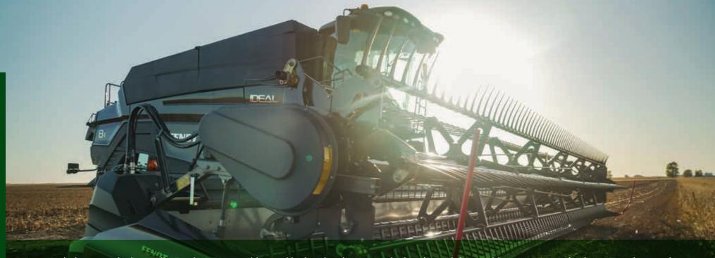
An industry exclusive to the Fendt IDEAL combine and its headers is our AutoDock™ system. With AutoDock, you can attach your Fendt header to the combine within five seconds, without ever leaving the operator's seat.
